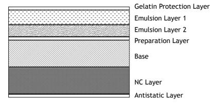
TIPS: The original "ATM 400" was coated onto a thinner film base than the standard 35mm films. It used a 65  $\mu$ m polyester base which is noticeably thinner than the new version coated on a 100  $\mu$ m polyester base.
